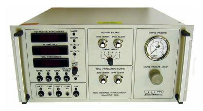
Fulfills THC requirements for 2. BlmSchV. 13. BlmSchV and 17. BlmSchV (DE) and fully complies with EN 12619 and EN 13526 (EU) and EPA Method 25A and Method 503 (USA)
